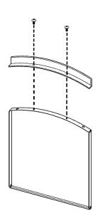
20. Second, attach side burner tray to side burner base using (4) #10 x 1/2" screws holes as shown. (SEE FIG "B")
